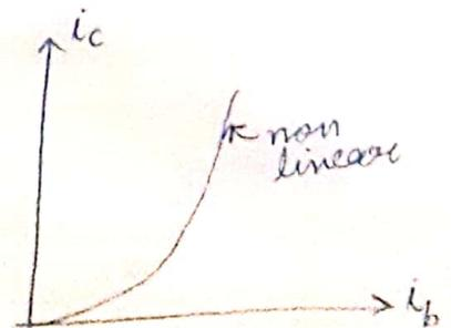
$i_b = I_{Bm} \cos \omega t$  (O/P signal which is assumed that cosine in nature).
