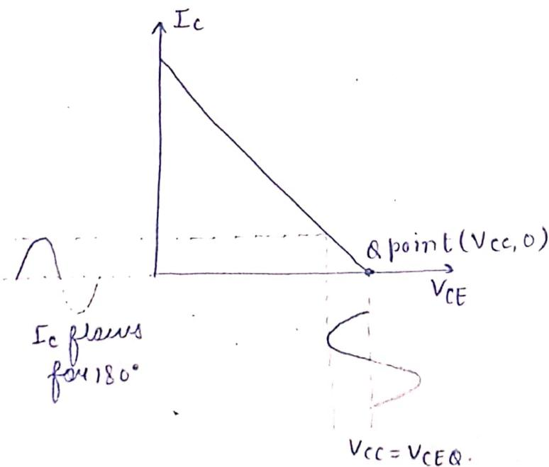
→ for +ve cycle, Tx is in active region & for -ve cycle Tx enters into cut off region.
