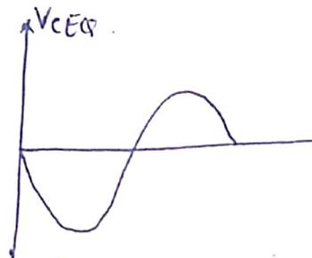
Phase of  $V_{CE}$  is change because it is Reverse battery which is connected in output side.
