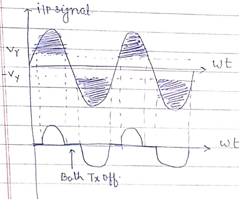
→ Hence there is a period b/w crossing of half cycle of i/p signal for which both Tx are cut off. Hence o/p signal get distorted.
