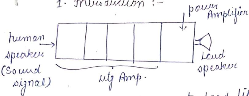
• Input stage & all intermediate stages are ~~its~~ small signal Amp<sup>s</sup> and use to increase the gain of Amplifier. It is called utg. Amplifier.
